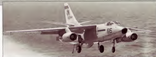
Above: With its landing gear and tailhook deployed, this A-3B is just about to 'trap' aboard the USS Forrestal. The weight of the A-3 meant that the arrestor gear had to be very strong.
